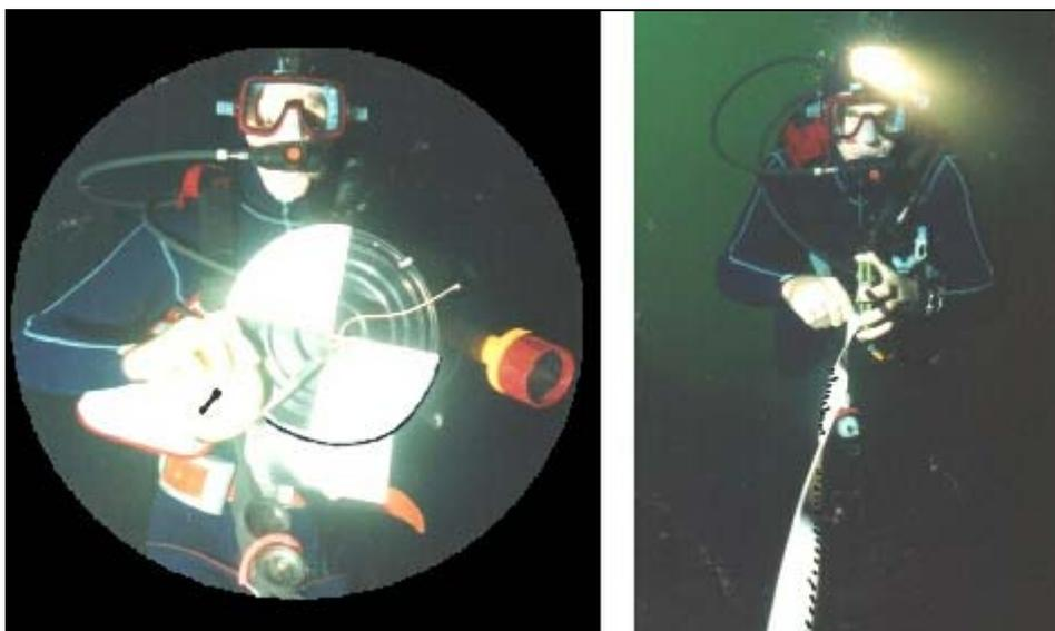
Using a Secchi Disk to Record Visibility Differences
