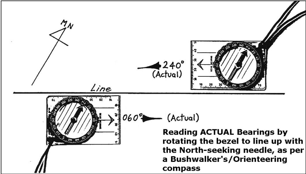
**Reading ACTUAL Bearings by rotating the bezel to line up with the North-seeking needle, as per a Bushwalker's/Orienteering compass**
